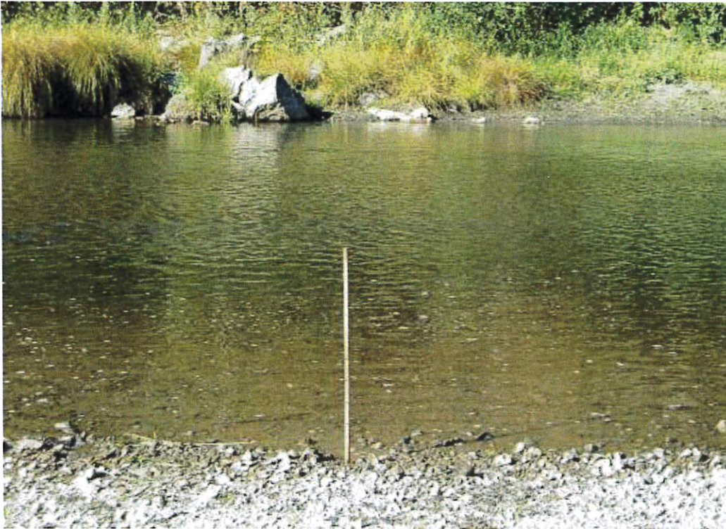
Figure C-1. Cross-section #1. Water surface elevation changed \approx 2 inches. Width changed 2.2 ft out of \approx 80 ft (2.7 %).
