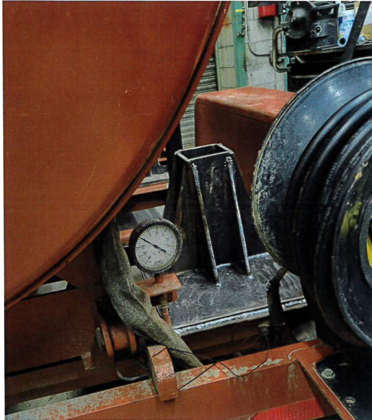
Mounting bracket installed
