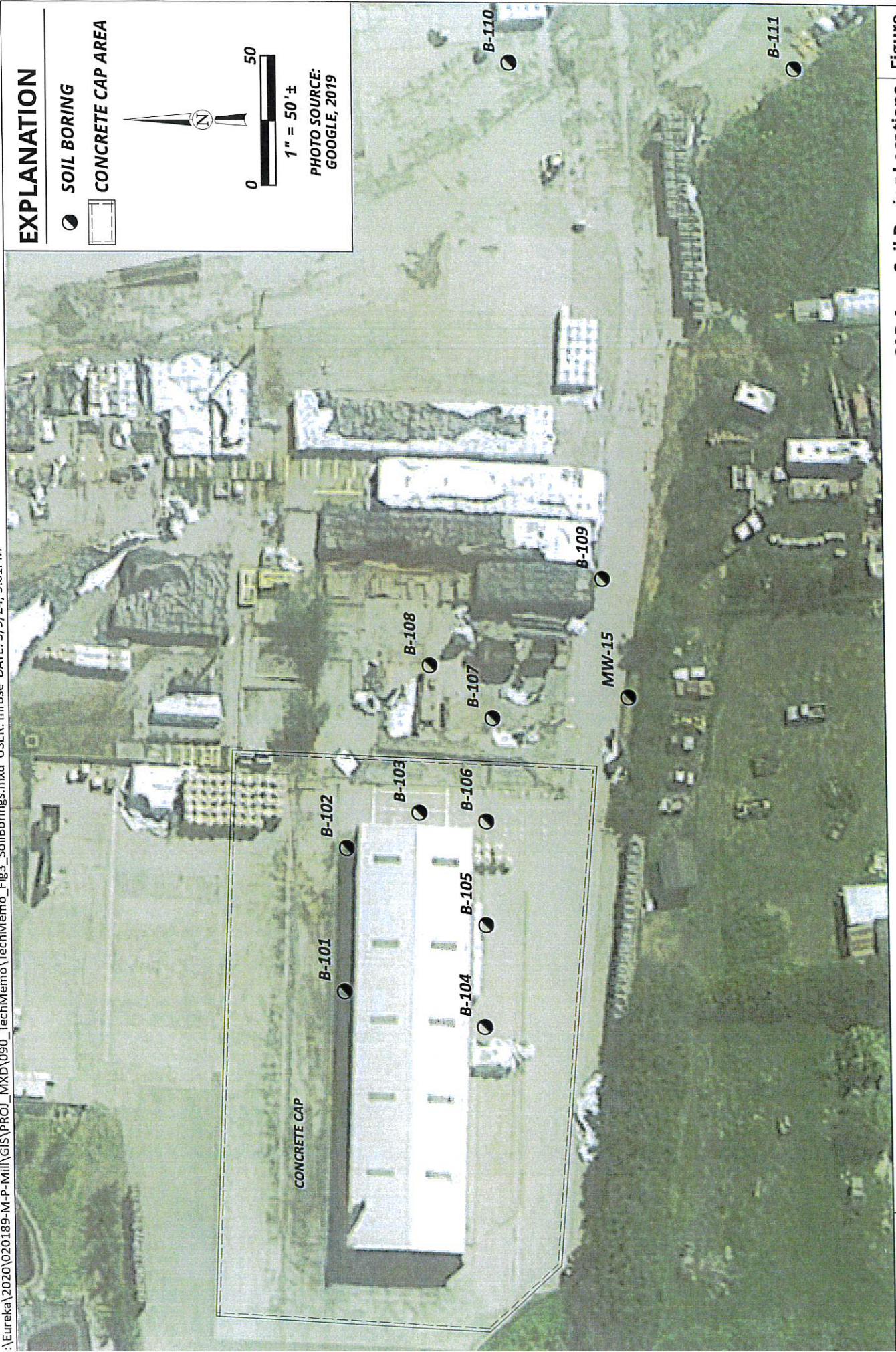
EXPLANATION ● SOIL BORING ▭ CONCRETE CAP AREA 1" = 50' ± PHOTO SOURCE: GOOGLE, 2019 Figure 3 CAP Area Soil Boring Locations May 2024 - 020189.090 Former McNamara & Peepe Lumber Mill Technical Memo 1619 Glendale Drive, Arcata, California
